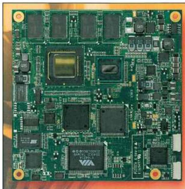
The conga-CA which utilises the Intel Atom Z5xx and US15W system controller hub.
